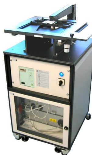
System for automated SCAN x-y-scanning table (left) / Spectrometer and light source rack excluding operating PC with manual LAB x-y-table (right)
