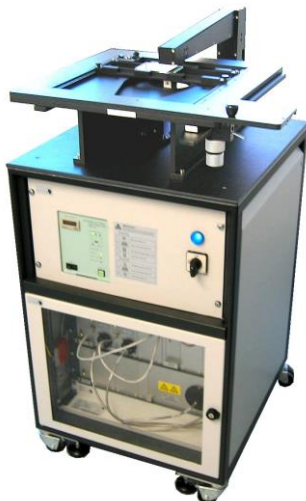
Spectrometer and light source rack with manual x-y-table (Xelas LAB)
